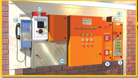
The Call Bell Unit (9) is an emergency signalling unit as required by the MHSA Reg 16.43.6 and is designed with two buttons both behind a breakable glass. One button to be used for accident to person, the other for an accident to shaft, both signals are followed by a station ID. An option to trip the winder after activating the accident to shaft button can be included.
