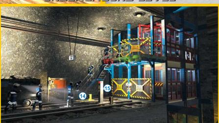
Deebar, known for its shaft safety products in mining, designed and manufactured the Deebar Slam-It, Slide-it, Lock-it and Latch-it Station Gate Lock (13) which is specifically designed to prevent a double operation and can, in addition, be electrically interlocked to the winder safety circuit via the integrated interlocking magnetic switch utilizing RS 485.
