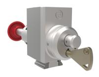
S40 IR Escape Release Adaptor module is used in conjunction with a releasing amGardS40 unit, to provide an escape function from an interlocked hazardous area. There are three versions, one with a key reset, one with a push button reset and one with a simple pull reset. The other option is the length of plunger needed to clear the door post thickness. This unit must always be mounted as the first module under the head.
